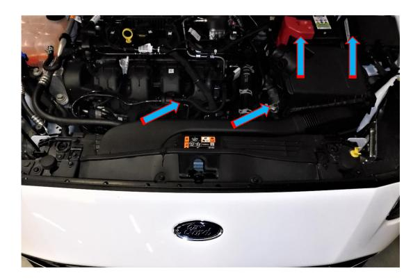
6. Release the hose clamp attaching the rubber hose to the diverter valve. And remove the hose completely.
