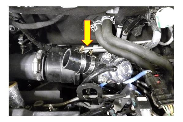
11. Using a 7mm socket and ratchet secure the supplied silicone hose reducer to the plastic boost pipe with the supplied 60-80 hose clamp. Place the 70-90 hose clamp loosely
