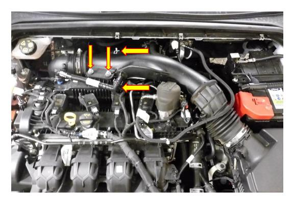
3. Using a 7mm ratchet and socket remove both hose clamps at each end of the intake pipe. You will now be able to pull the intake pipe out of the engine bay.
