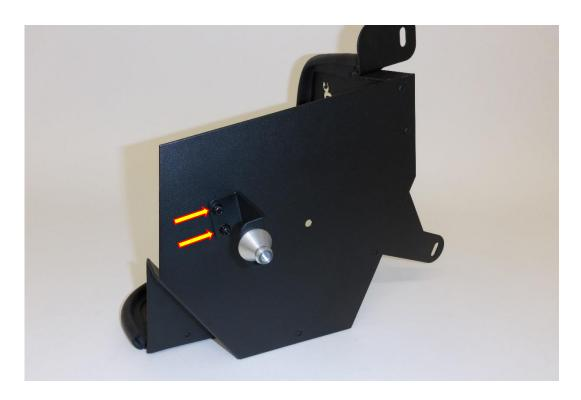
Using a 10mm spanner attach the billet mounting peg to the bracket using the supplied M6 fastener and washer.
