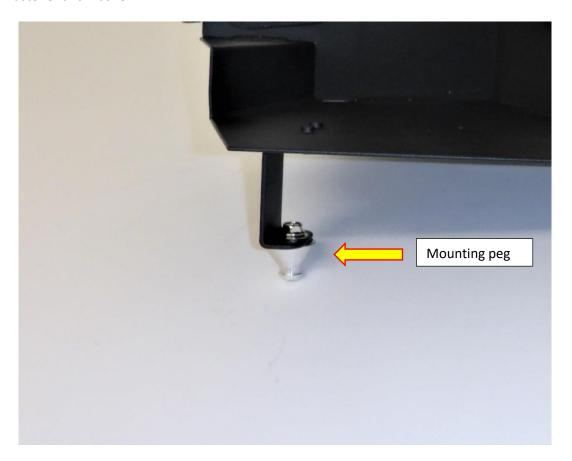
8. Fit the filter tray into position, the mounting peg will push into position the other two mounting points are attached using the M8 nut, bolt and X2 washers per mounting point. Look at the picture below which shows how it should be mounted.
