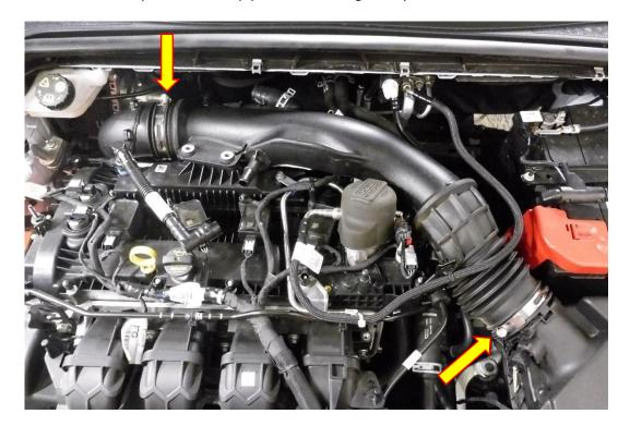
4. Twist the MAF sensor anti clockwise to allow you to remove it from the airbox.
