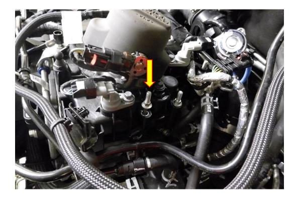
**10.** Using a 7mm socket and ratchet secure the supplied 25-45mm hose clamps and silicone hose to the diverter valve output.
